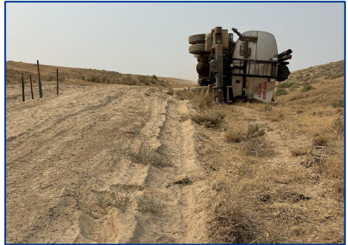
The T-posts (on left) that the water tender operator tried to avoid by driving over onto the soft moon-dust shoulder—and the vehicle slowly tipped over.
